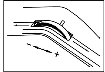
Releasing the trigger approximately one or two inches prior to the completion of the cut will help keep the blade clean and free from buildup. Never use a metal bar as a guide. If the blade touches the metal guide the heat from the blade will be dissipated by the metal guide. This will lower the heat of the blade and affect its cutting quality.
